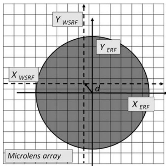
**Figure 1.** Wavefront sensor reference frame (WSRF), and eye pupil reference frame (ERF).
